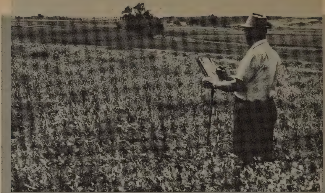
A soil scientist in the late 1950s sketches soil type boundaries on an aerial photograph after making ground probes.
